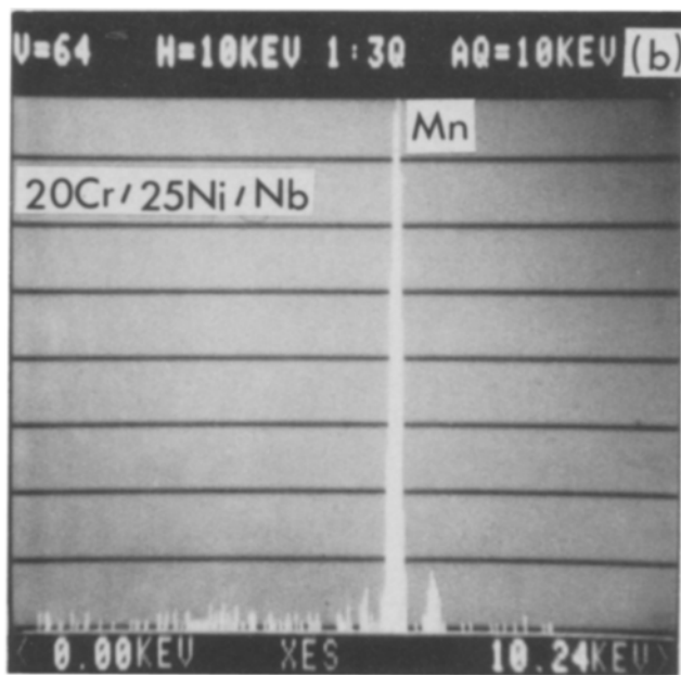
Figure 1 "Radioactive" EDX spectra from samples of neutron-irradiated (a) PE16 and (b) 20Cr-25Ni-Nb. Both were collected with the electron beam switched off. They contain characteristic manganese X-ray peaks on a background distribution.
