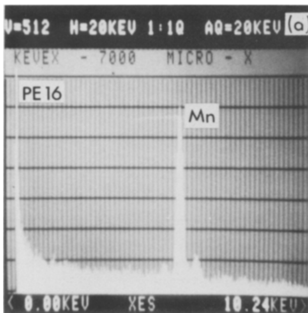
Figure 1 "Radioactive" EDX spectra from samples of neutron-irradiated (a) PE16 and (b) 20Cr-25Ni-Nb. Both were collected with the electron beam switched off. They contain characteristic manganese X-ray peaks on a background distribution.
